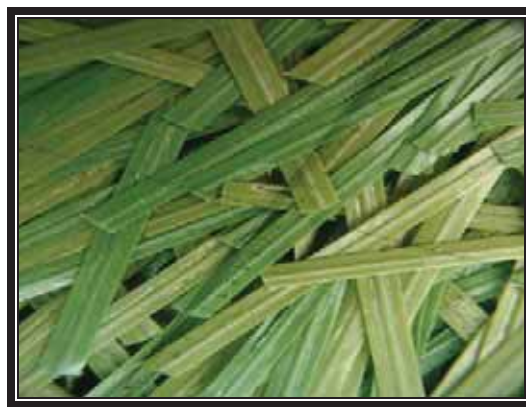
Tencate Yarn after 12,000 cycles of Lisport Test Method
